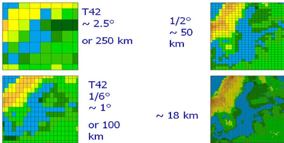
Fig. 1 A model domain in the Baltic Sea with the terrain at different spatial resolution from a coarse global climate model (upper left) to a higher resolution regional climate model (lower right).
